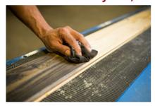
All Synergy Wood products are made with tongue and groove joints. Tongue and groove is the preferred method of fitting our wood boards together, edge to edge. Tongue and groove joints allow two wood planks to be joined strongly together to make a single flat surface and conceal the effect of wood shrinkage. "Tongue and groove" is often abbreviated as T&G.
