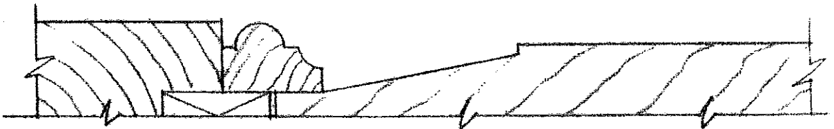
B&S M-132 (1/2" x 3/4") INSET MOULDING; PARTIAL RAISED PANEL
