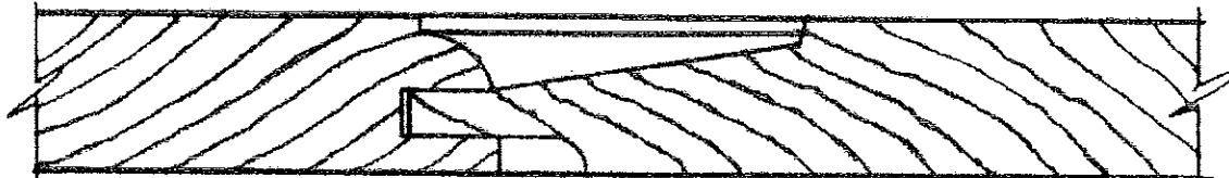
3/4" THICK DOOR; 3/4" THICK RAISED PANEL
